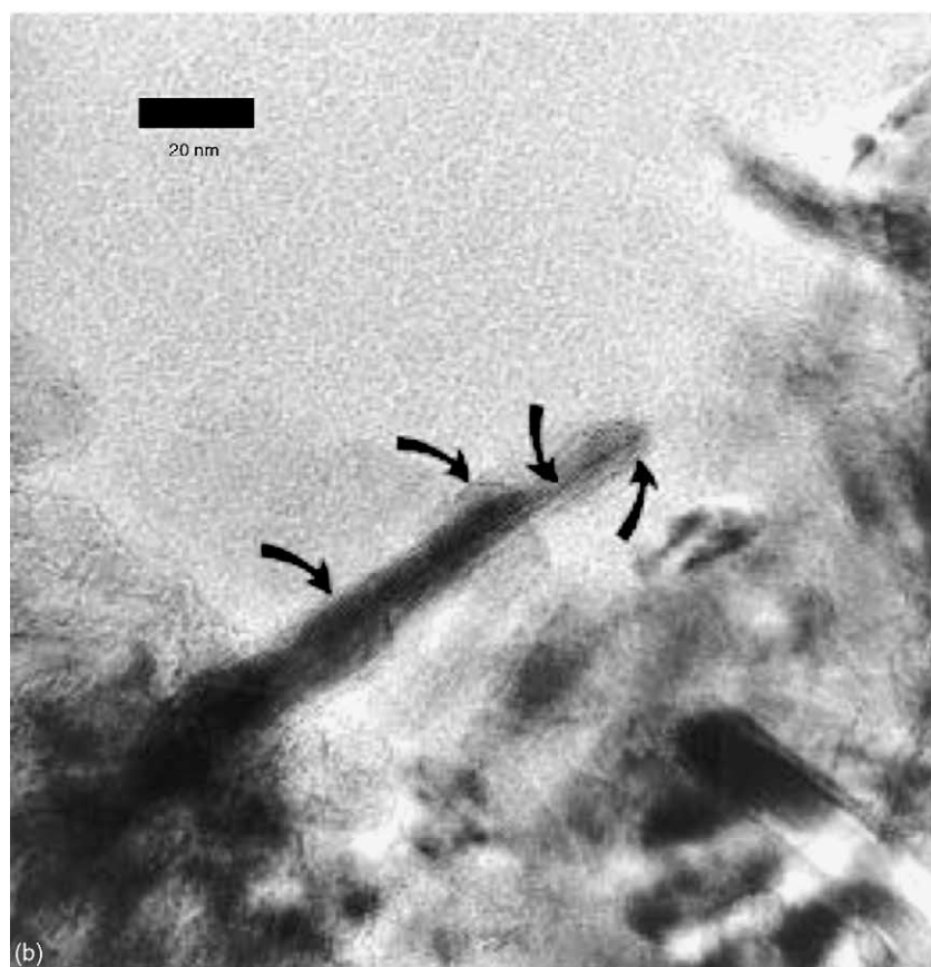
Fig. 7. HREM micrographs of NiMo/Al 2 O 3 -MgO (1.0) catalysts: (a) sulfided after recent preparation; (b) and (c) sulfided after 6-months exposure to ambient conditions.
